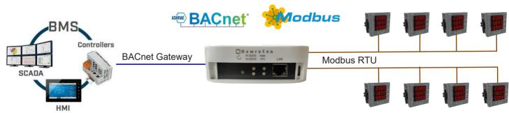
To communicate to multiple Modbus RTU devices at the same time across a RTU network. Only chosen points can be read from multiple Modbus RTU devices by BMS as a single BACnet IP device
