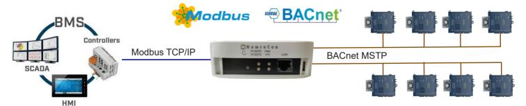
To communicate to multiple BACnet MSTP devices at the same time across a MSTP network. Only chosen points can be read from multiple BACnet MSTP devices by BMS as a single Modbus TCP/IP device
